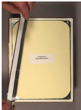
Foil tape shown prior to positioning onto glass and around copper tray
