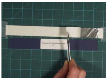
Liner is pulled off to expose the tape adhesive
