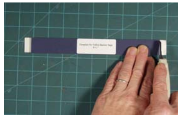
Liner is cut through without cutting foil tape: at both ends of tape
