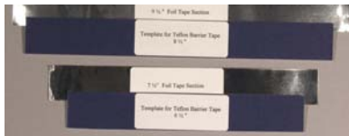
Pre-cut foil tape sections with templates for cutting liner:
