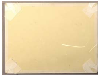
Reverse of plate package with the Teflon attached to Mylar backing sheet
