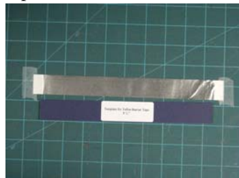
Liner is cut through without cutting foil tape: at both ends of tape
