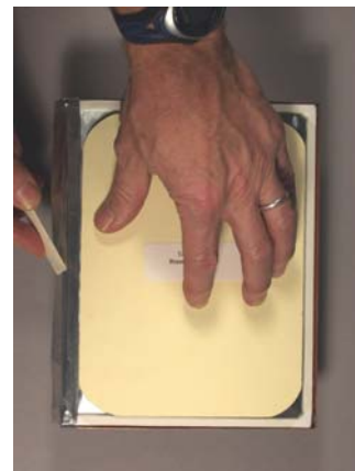
The corner sides are carefully pressed down to the copper and burnished
