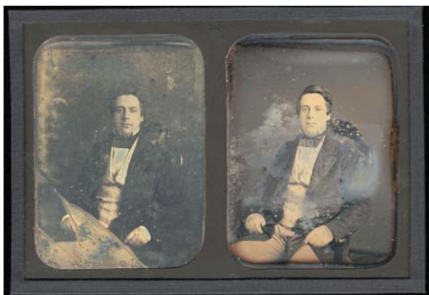
Fig. 74: Example of tarnished area on daguerreotype due to previous broken cover glass
