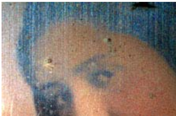
Fig. 58: Vertical polish marks on stereo daguerreotype plate
