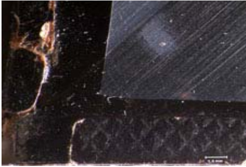
Fig. 83: Failed binding tape
