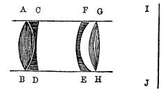
The achromatic lense is composed of two pieces, crown and flint glass, cemented together, the crown glass A B, is double convex, and the flint glass C D, double concave. The flint glass has a greater dispersive power than the crown glass, and its refraction being in an opposite direction it corrects the aberation of
