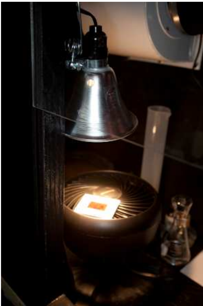
Fig. 8 - Becquerel development setup
