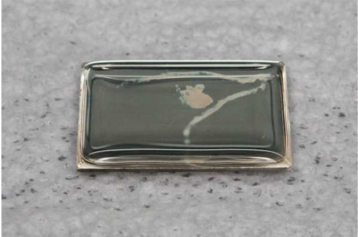
Fig 9 - Cold gilding a plate
