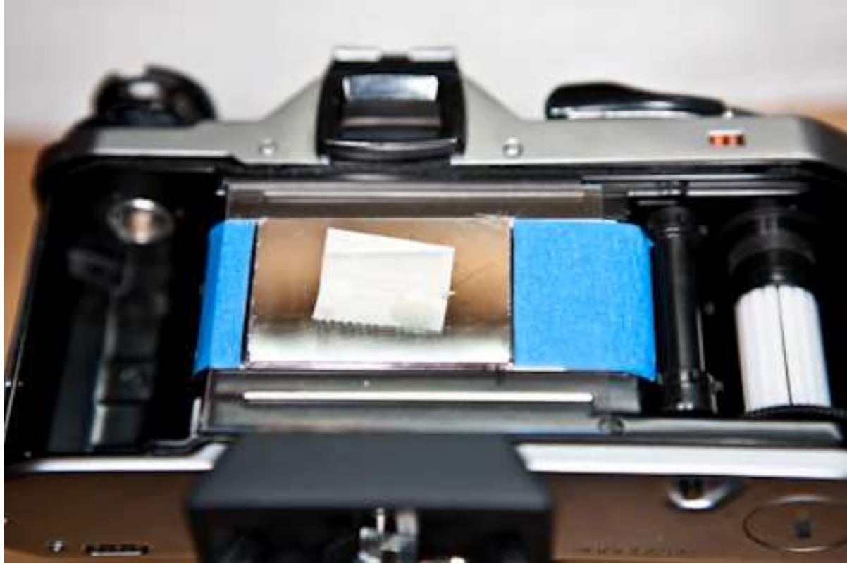
Fig. 7 - Camera with polycarbonate plate guide and plate
